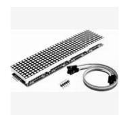
It provides I2C reception of up to 128 ASCII characters and displays on a set of 8\*8 matrices connected in series horizontally, through a Max7219 circuit for each of them.
